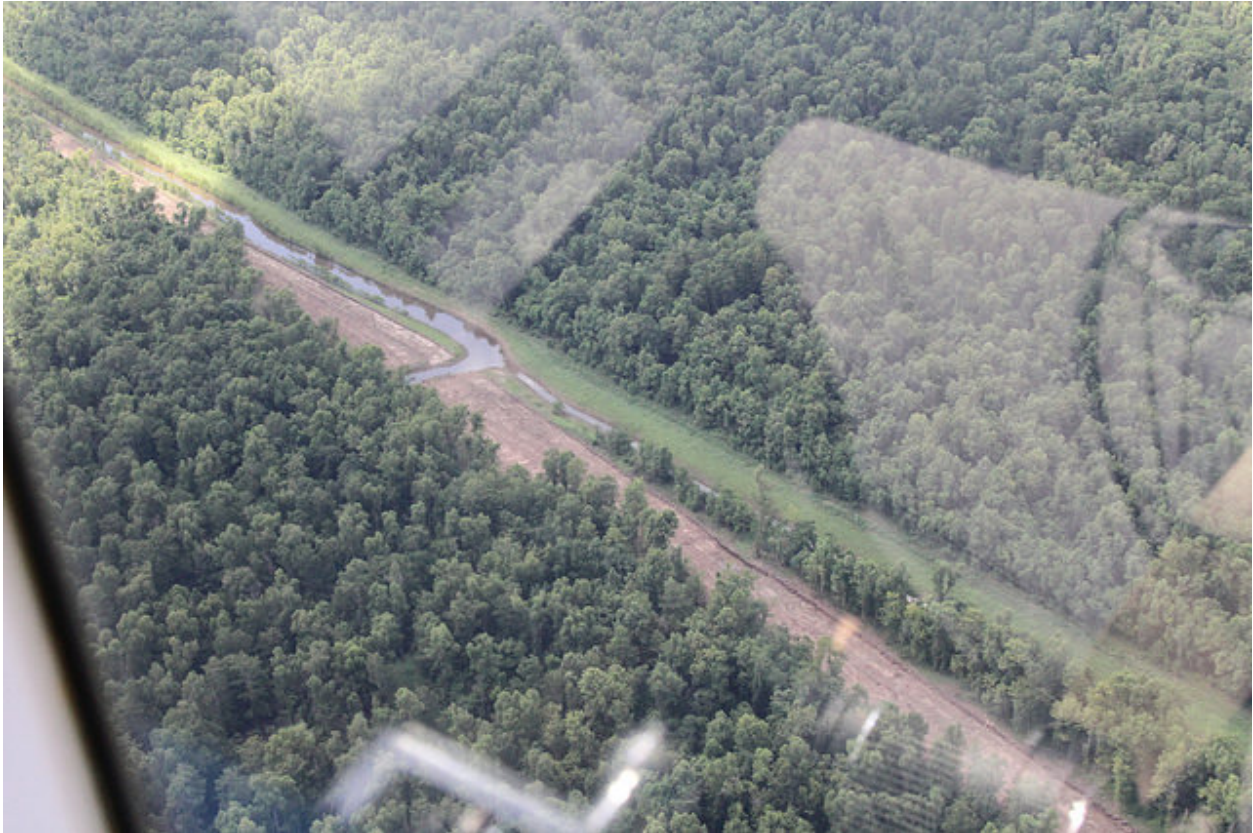
Figure 2. This photo was taken by Scott Eustis of Gulf Restoration Network during a monitoring flight on June 28, 2018. This photo depicts the pipeline right of way as it crosses the Property. As seen in the photo, the right of way has been cleared of trees.
